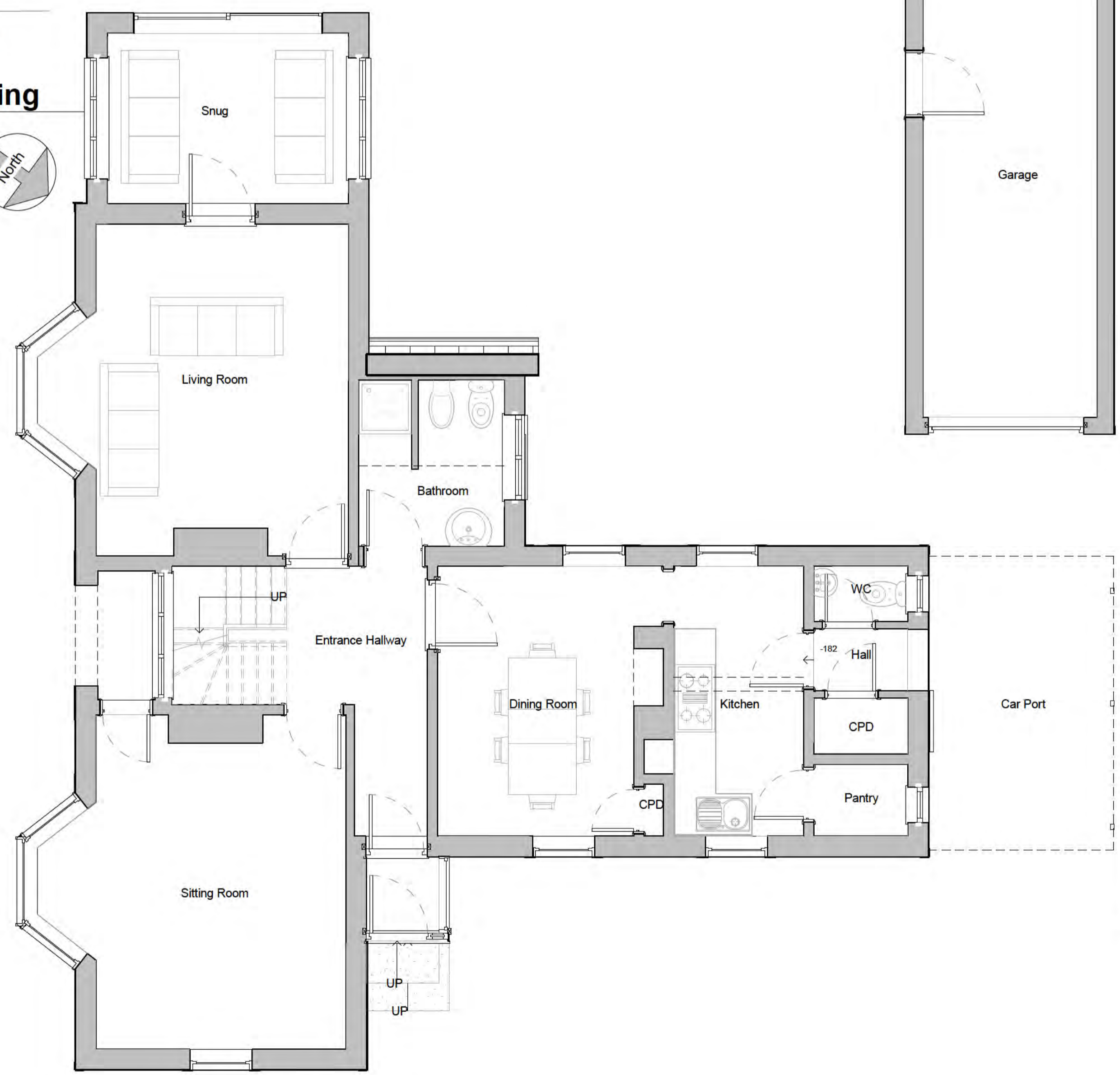
3 Ground Floor - As Existing 1 : 50
