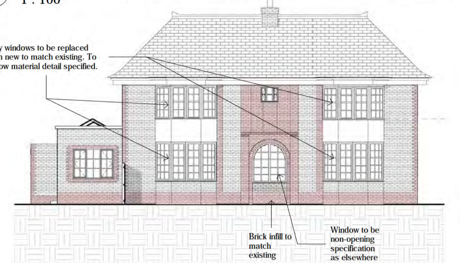
7 Side Elevation SE - As Proposed 1 : 100
