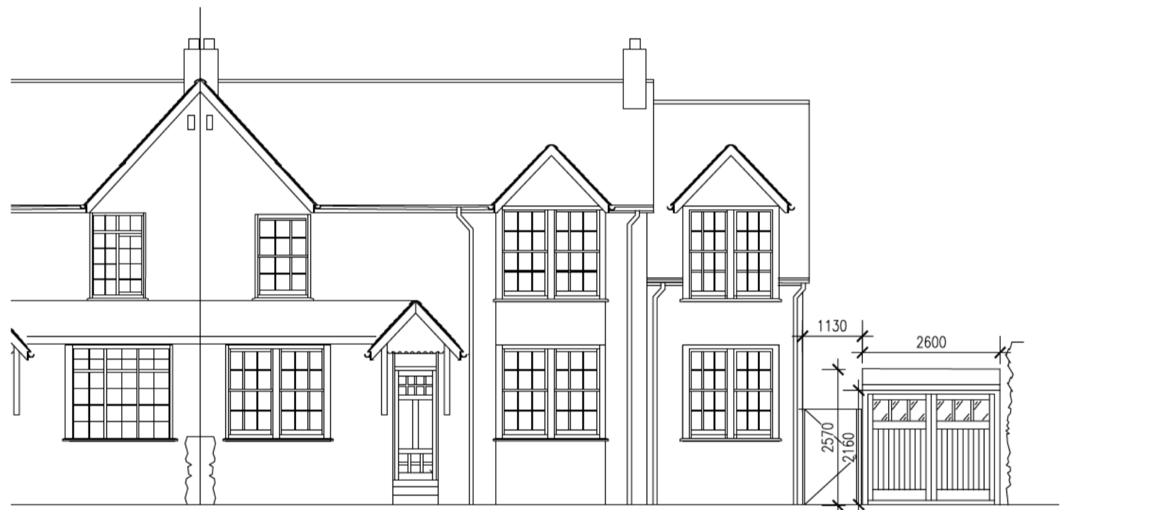
04 Front Elevation as Existing 1:100
